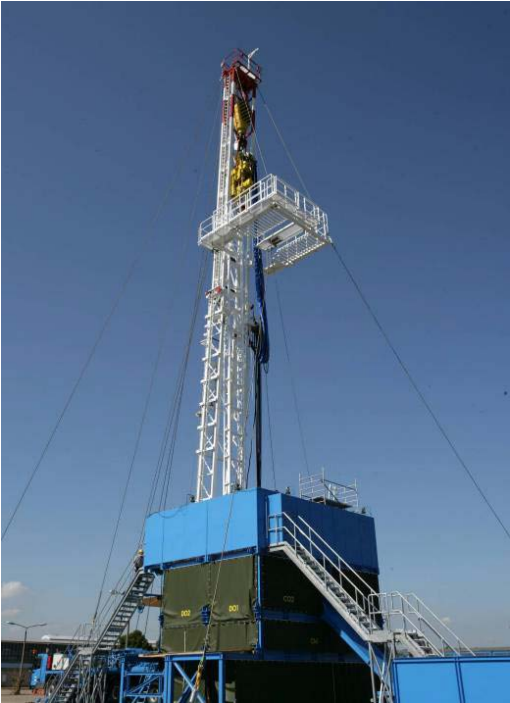
Working platform and monkey board
